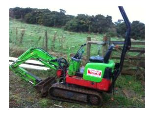
It was completed over two days with a mini digger and recycled plastic tube from the bail wrapping. This acted as a duct or sleeve to thread the poly water main through once dug and backfilled with sand and muck.
